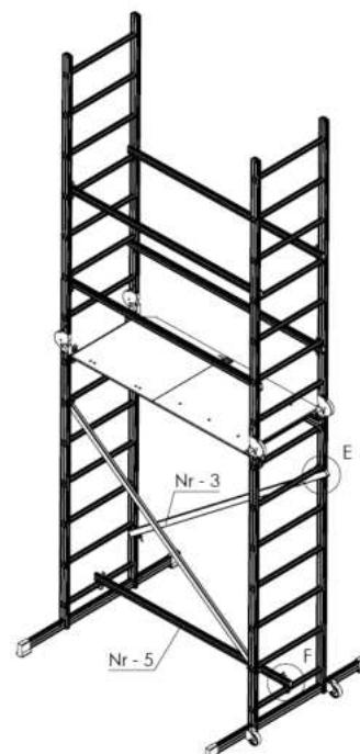
**EN / Mount the struts under the platform:** in platforms mounted below the maximum height.
